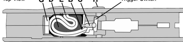
(5 Carefully remove battery clip (E) from old battery and place it on new battery. NOTE: battery terminals only fit one way in clip.
