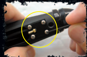
Remove Rear Air Barb Block
