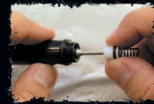
Remove Poppet & Valve Spring
