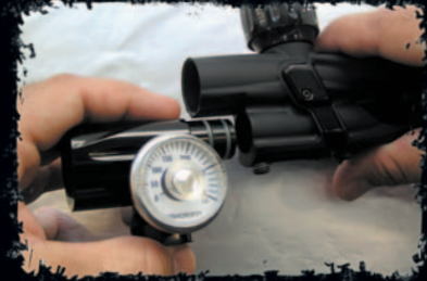
Remove ASA Block From Body
