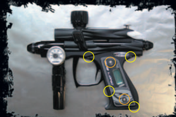
2 Open Trigger Frame
