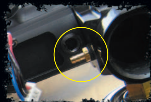
Remove Air Barb From ASA Block
