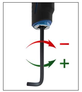
You can adjust your velocity through the Hyper6s Pro™ regulator, located in the fore grip. To adjust the velocity, insert a 3/16" Allen wrench into the bottom of the fore grip. Turning the Allen wrench clockwise, or in, will lower the output pressure, decreasing the velocity. Turning the adjustment screw counterclockwise, or out, will raise the output pressure, increasing the velocity.
