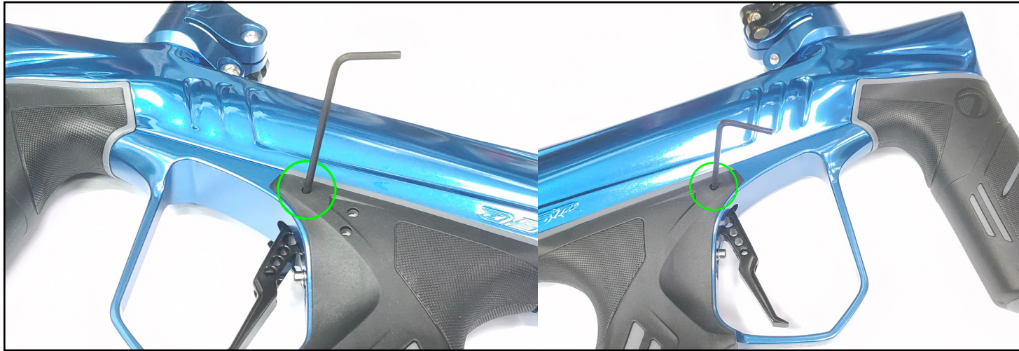
1. Use a 5/64" Allen wrench to remove the screw located at the top front under the grip.
