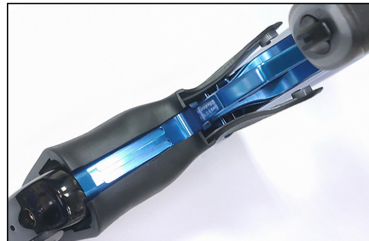
4. In doing so, you will have released the last three locking tabs that are under the molded finger grooves.
