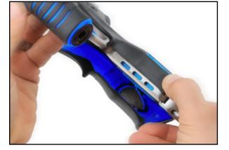
6. In doing so, you will have released the last three locking tabs that are under the molded finger grooves.
