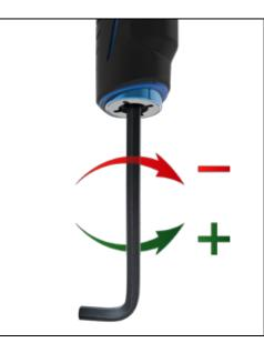
You can adjust your velocity through the Hyper6s Pro<sup>™</sup> regulator, located in the fore grip. To adjust the velocity, insert a 3/16" Allen wrench into the bottom of the fore grip. Turning the Allen wrench clockwise, or in, will lower the output pressure, decreasing the velocity. Turning the adjustment screw counterclockwise, or out, will raise the output pressure, increasing the velocity.
