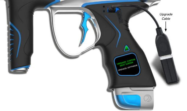
You can customize the boot screen on your M3+ with any photo you like. The full color provides remarkable detail and image resolution. **Before you can download a photo onto the board it will first need to be converted to a .bmp file sized 128 x 128 pixels**. You can use any number of online programs. Depending on converter used, Bit Depth or color should be set at 24 (true color).
