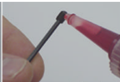
7. Using the medium bottom body screw supplied, apply red loctite and insert screw into underside of body. Screw in snug, but do not over-tighten. Over-tightening could damage the tapeworm.
