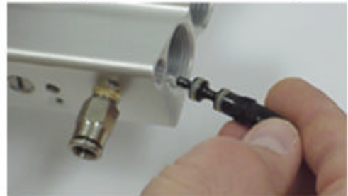
5. Insert tape worm into front air chamber hole. (Make sure both o-rings on tapeworm are greased for installation.)
